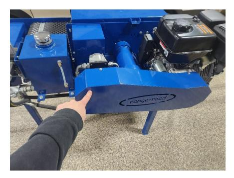
Main Belt cover – all the drive belts for the blades AND the belt that drives the hydraulic pump are behind this cover.
