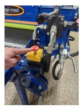
The emergency kill switch. if it is pushed down, it must be twisted to pop back up. No spark when switch is depressed.
