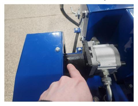
There is a grease fitting on the back bearing housing – ensure this is greased daily.
