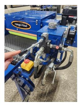
This Hydraulic control lever is used to operate the main belt.
