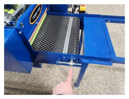
There are four of these "bolt" adjusters on the unit, 2 at each end of the main belt. They are used to add or reduce tension on the belt – they come pre adjusted from the factory. Only adjust if your belt is slipping or is running un-even.
