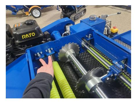
There are 6 of these roller adjustment bolts on the machine – 3 on each side.
